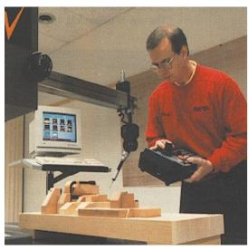
Brown & Sharpe's horizonal 2000 CMM measures a tubular checking fixture in about one-fifth the time it formerly took using a height gage. One specialized measurement program can be used to measure a multitude of dimensionally different tubular checking fixtures.
