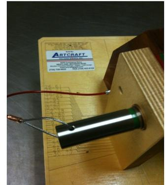
ArtCraft's gages are all designed using computer aided design software. All the gage components are laid out on the gage base and blocks using a patented CNC laser process that "laser scribes" all the lines and dimensions to very close tolerances (not laid out by hand).
